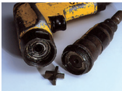
Damaged pneumatic tooling
